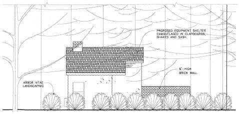
This equipment shelter, to be built in New England, will be camouflaged as a New England Cottage with clapboards, shakes and sash.
