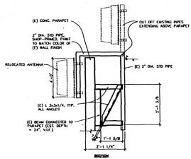
Panel antennas should be located so that they do not peak above the roofline and should be positioned below the parapet, as shown in this drawing from GEZ Architects Engineers.
