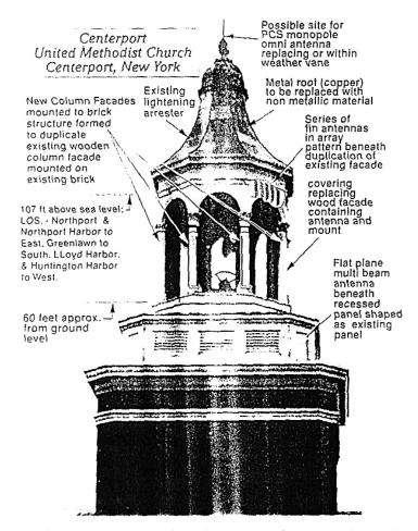
This is a proposed tri-location of personal wireless service facilities on a landmark church in Centerport, New York. Proposed design courtesy of GEC-Marconi Hazeltine.
