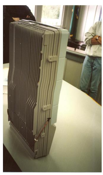
This is a microcell. It is well designed because it is small. It could be located anywhere and sited almost anywhere.
