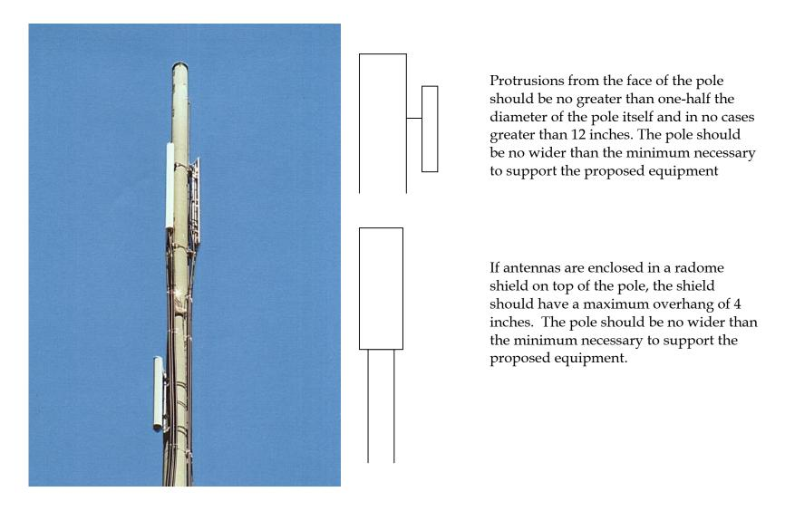
Personal wireless service facilities are composed of antennas and equipment. The equipment is housed in equipment shelters, cabinets and areas that should be small and designed to blend with the surrounding environment or buried underground. The County recognizes that differences exist between Cellular Analog, Cellular Digital and PCS equipment. Each system should use the smallest equipment available and use sites and designs that minimize the equipment's impact.
