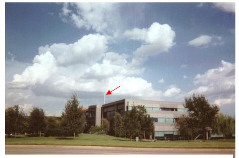
This omnidirectional antenna is part of a personal wireless service facility that is camouflaged as part of the GTE Headquarters in Irving, Texas. It could also be considered disguised as a flagpole, but it does not function as a flagpole.
