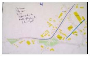
Figure 14 3) Hydraulic under 29; 4) Continuous flyover from Hydraulic to Barracks w/center ramps
