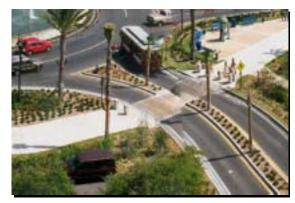
Figure 50 Median splitter islands and set-back crosswalks create safe pedestrian crossings
