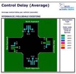
Figure 49 SIDRA analysis shows capacity, delay, and levels of service for roundabouts
