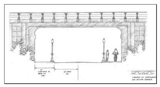
Figure 43 Cross section of Angus Road Underpass
