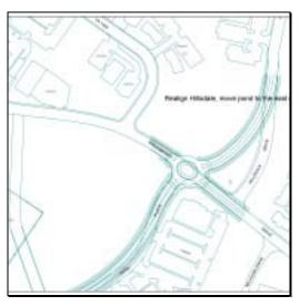
Figure 33 The northern end of Hillsdale Drive Extended could be realigned with a roundabout at the intersection with Greenbrier to improve traffic flow and turning movements
