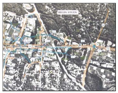
Figure 28 Rt 29 Pedestrian Study identified priority sidewalk connections
