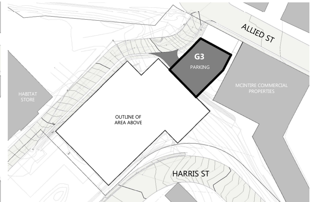
G3 PARKING; BY RIGHT ACCESS FROM EXISTING DRIVEWAY AT ELEVATION 413 APPROX 4,000 SF
